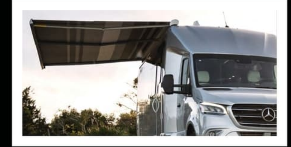
2 A powered, armless awning creates a wide exterior seating area.
