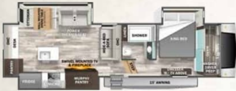
3125RD HITCH WEIGHT-2,050 lb. / GVWR-16,050 lb. / UVW-11,609 lb. CCC-4,410 lb. / LENGTH-35' 7" / HEIGHT-13' 6" / WIDTH-96"
