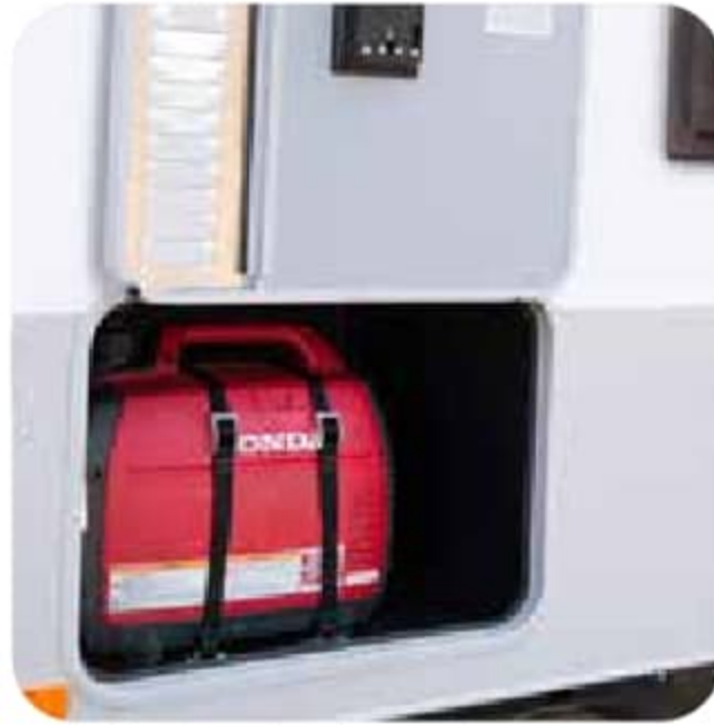
Portable Generator Storage Compartment W/Tie-Downs
