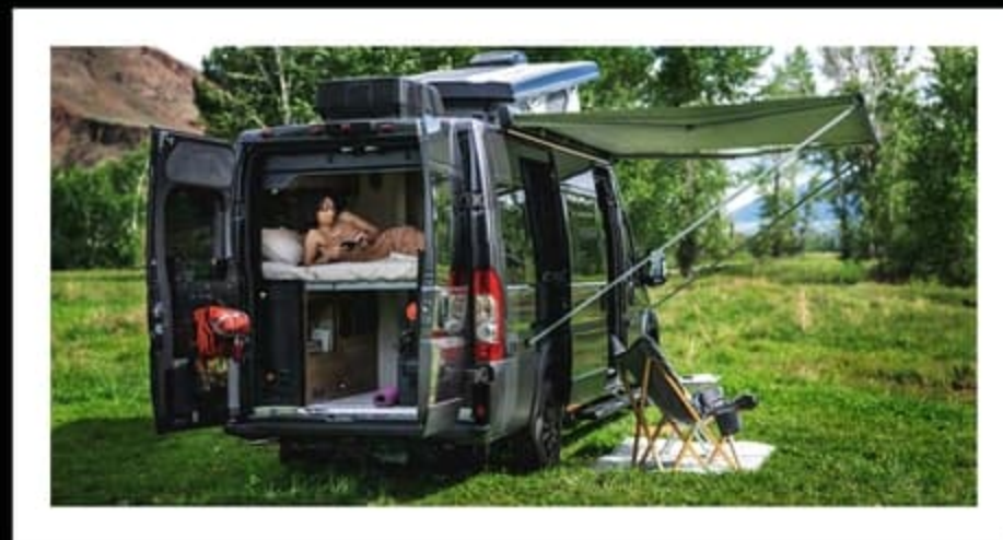
6 A 12-foot awning with legs expands to create a shady exterior living space.
