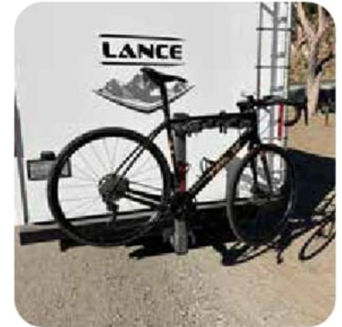
2" Utility Receiver. Standard receiver hitch for bike or storage racks. Limit 300 lbs. capacity.
