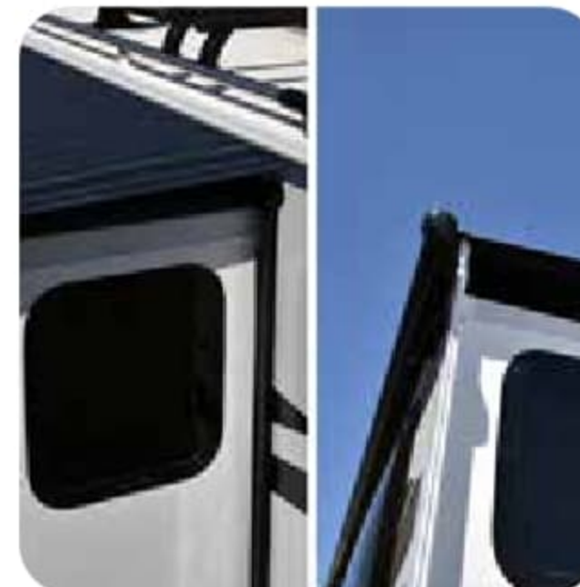
Awning Slide-Out Cover(s). Keep debris off the roof; any debris that falls onto the topper tends to slide off easily.
