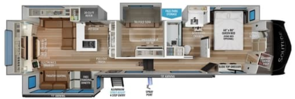
388MBS UVW 1 15,600 HITCH 1 2,900 GVWR 19,000 LENGTH 1 42' 11" HEIGHT 1 13' 5" CAPACITY 83 106 53
