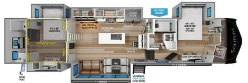
391DL UVW 1 15,500 HITCH 1 3,100 GVWR 19,000 LENGTH 1 42' 5" HEIGHT 1 13' 5" CAPACITY 83 106 106
