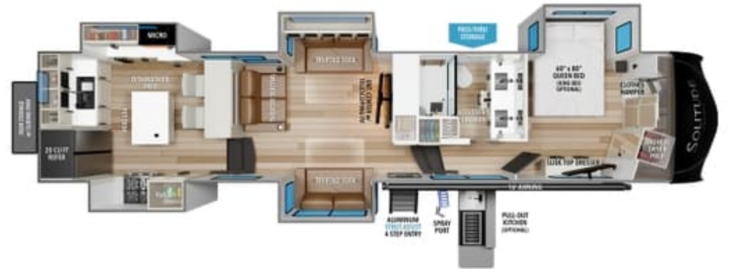
390RK UVW 1 15,000 HITCH 1 2,794 GVWR 19,000 LENGTH 1 42' 5" HEIGHT 1 13' 5" CAPACITY 83 106 53
