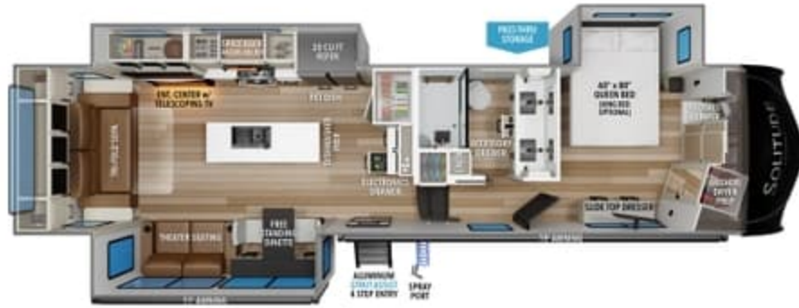
310GK UVW 1 12,500 HITCH 1 2,350 GVWR 19,000 LENGTH 1 34' 4" HEIGHT 1 13' 5" CAPACITY 83 106 53
