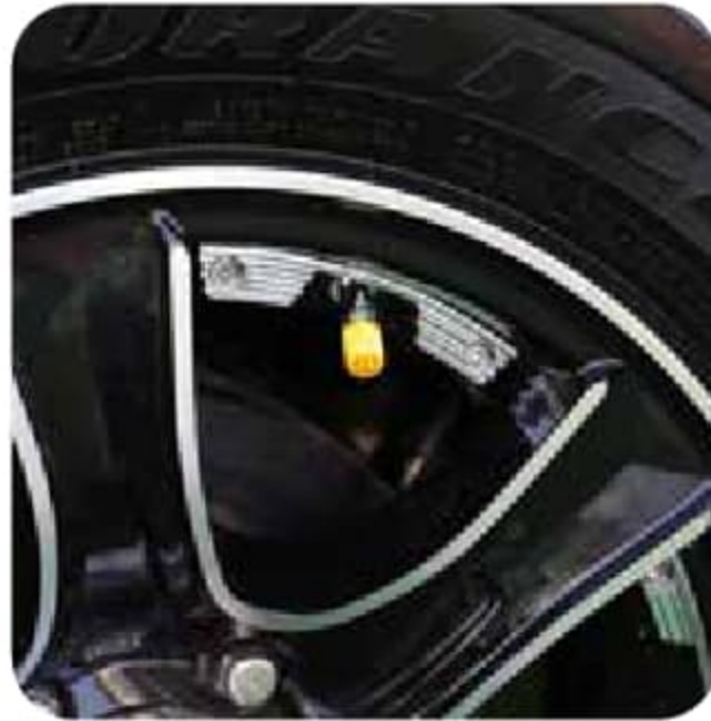
TPMS System (Tire Pressure Monitoring System). Monitor the pressure (PSI) in all four tires while going down the road.
