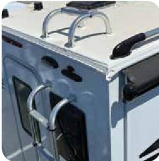
Ladder & Maggie Rack. Gain entry to your roof with this heavy duty ladder and a place to mount cross bars.
