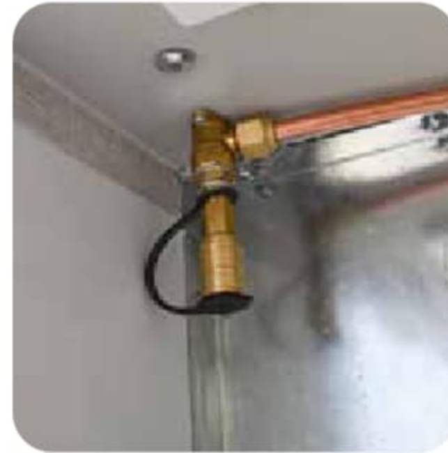
Exterior Propane Connection. Link into and draw from your onboard tanks for a BBQ or other accessory.
