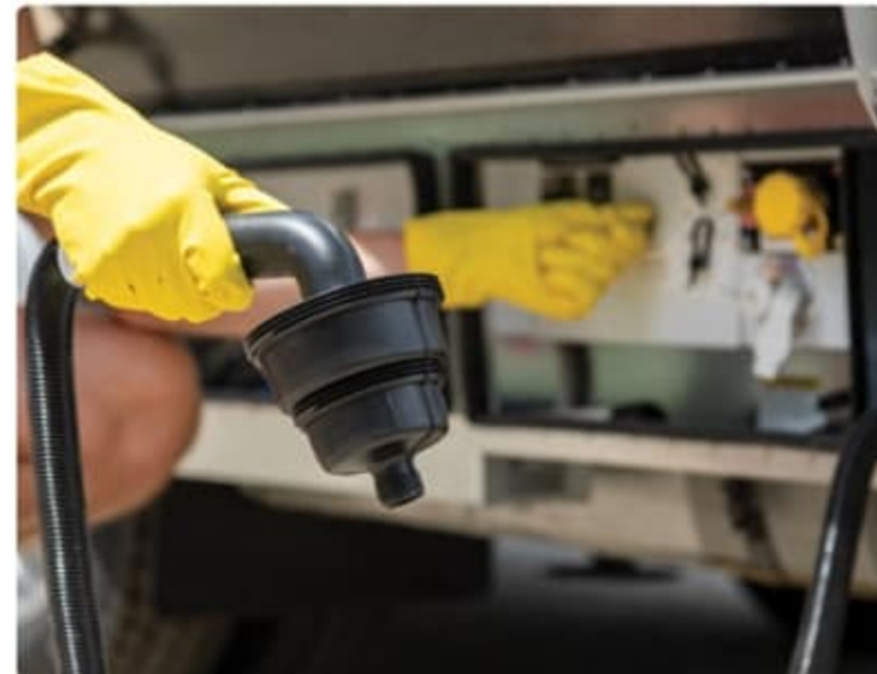
Macerator Sewage Discharge With Manual Disconnect
